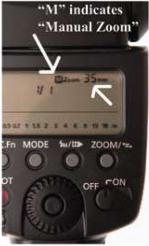
Image 2 - “M” stops zoom tracking. Set the angle of view on flash to 35mm.
