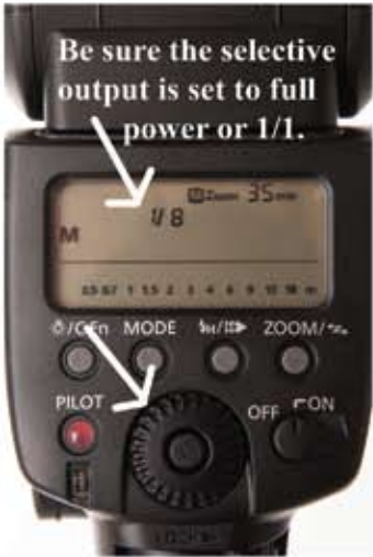
Image 3 - The selective output setting acts like a dimmer switch with lights in your home.
