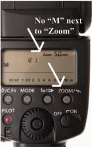
Image 1 - No, “M” indicates the zoom is automatically tracking the lens.
