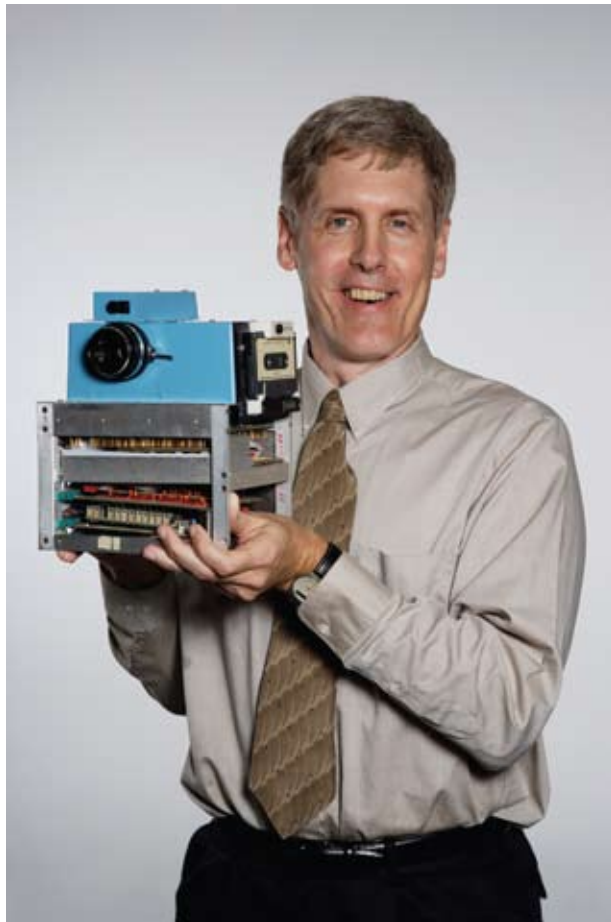
Steven Sasson with his first 0.01 megapixel digital camera, the size of a toaster; that produced a black and white image in 23 seconds back in 1975.
