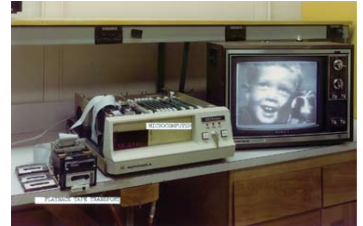
The “playback” system converted the data to a standard video signal that could be viewed on a television screen.
